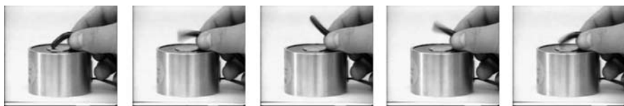
Fig. 28 Snapshot of shape change of a magnetoelast due to modulated magnetic field. The frequency of the field is 40 Hz
